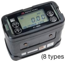
(8 types of gases detectable as standard)
