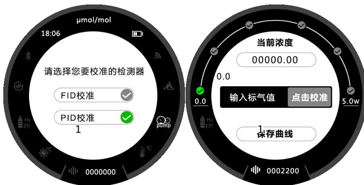
Figure 8-3 PID calibration diagram
