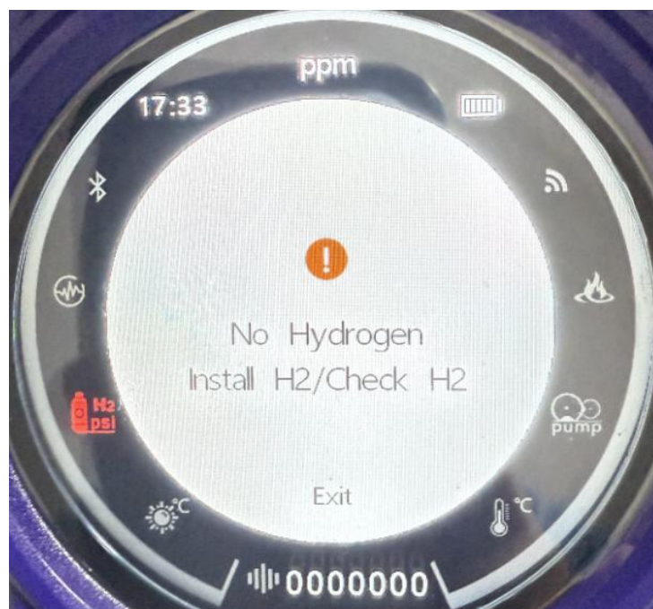
Figure 5-4 "No Hydrogen Source Detected" Alert Screen
